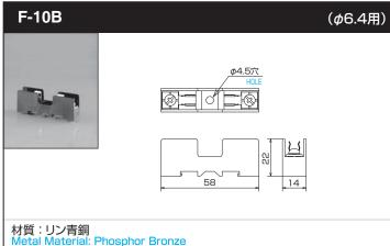
厚さ: 0.4mm Material Thickness: 0.4mm 仕上げ:ニッケルメッキ Finish: Nickel Plated 定格電流: 10A Rated Current 100 10A
