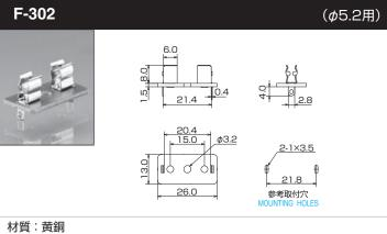
iterial: Spring Brass 厚さ:0.4mm Material Thickness: 0.4mm 仕上げ: ニッケルメッキ Finish: Nickel Plated
