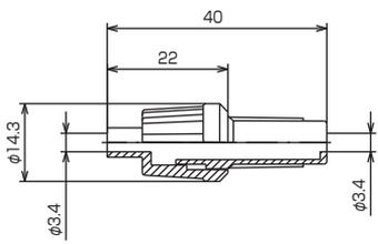
Dimensions: Total length 40, mounting length 22, diameter φ14.3, base diameter φ3.4, contact diameter φ3.4.
