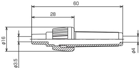
Dimensions: Total length 60, mounting length 28, diameter φ16, base diameter φ3.5, contact diameter φ4.
