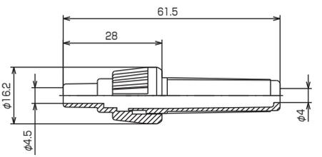
Dimensions: Total length 61.5, mounting length 28, diameter φ16.2, base diameter φ4.5, contact diameter φ4.
